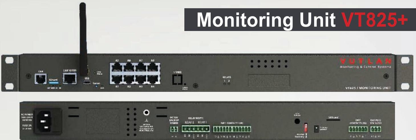
The unit is used in data centers, remote & industrial facilities, offices. Can connect up to 30 sensors, 12 dry contacts, two 12V alarm beacons, GSM modem, USB-cam, SD card, 1-Wire board (instead of VT18) for reader connection. There are built-in servers and agents like HTTP, HTTPS, SNMP v1, 2c, 3, SMTP, Radius, Syslog, FTP, DHCP, Watchdog.
